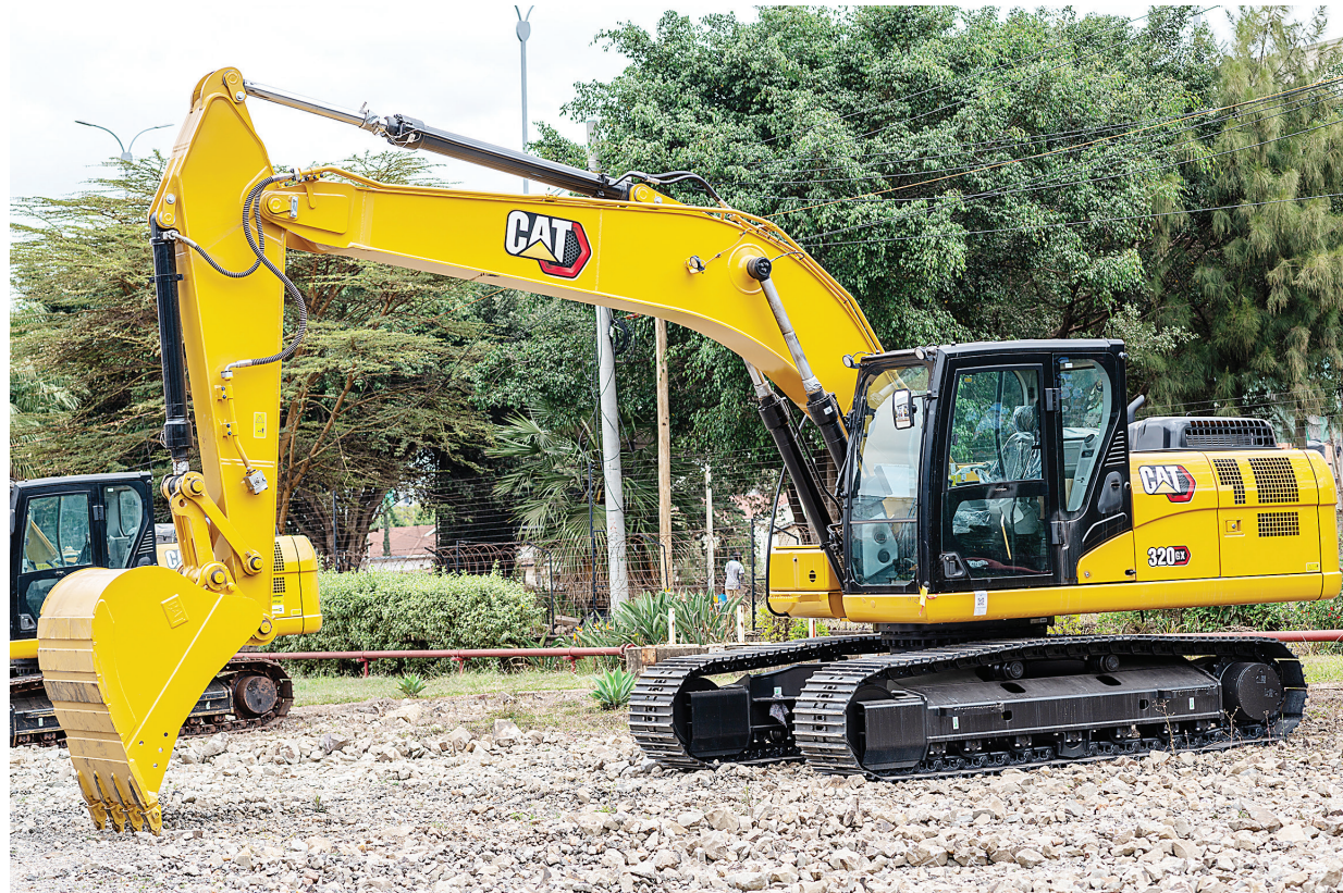
320 GX Hydraulic Excavator. PHOTO | MANTRAC KENYA
